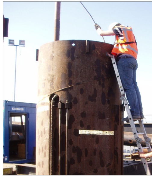
The SAAF being lowered into the pipe
