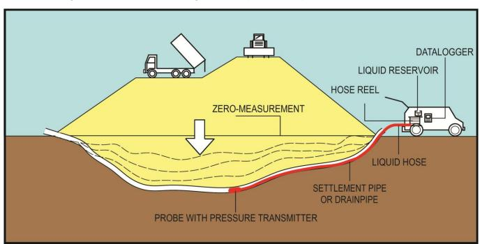
Contrary to other systems available on the market, the LPMH-system does not require that the pipe itself is filled with water: the LPMH-unit has its own liquid system. Whether the pipe is empty or wholly or partly filled with liquid (e.g. groundwater or drain water) does not make any difference for the operation of the LPMH-system.
