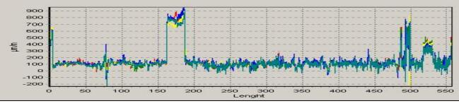
Soil deformation behind a quay wall
