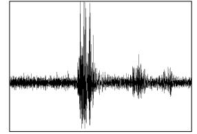
Audio wave form of a concrete lid being lifted
