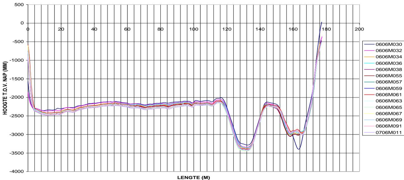
Contrary to other systems available on the market, the LPMH-system does not require that the pipe itself is filled with water: the LPMH-unit has its own liquid system. Whether the pipe is empty or wholly or partly filled with liquid (e.g. groundwater or drain water) does not make any difference for the operation of the LPMH-system.
