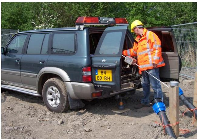
An important additional advantage of the LPMH-system in this particular case was that the measurements could continue after the construction was finished and the road had been taken into service so that any possible effects of the traffic load could be measured. These measurements were perfectly reproducible with the first (zero-)measurement at the start of the construction of the road.
