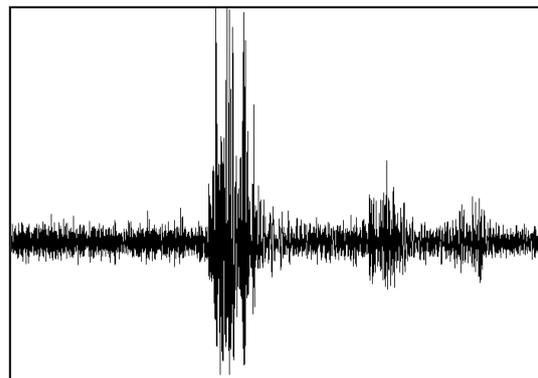
Audio wave form of a concrete lid being lifted
